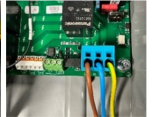
Single Phase Wiring
